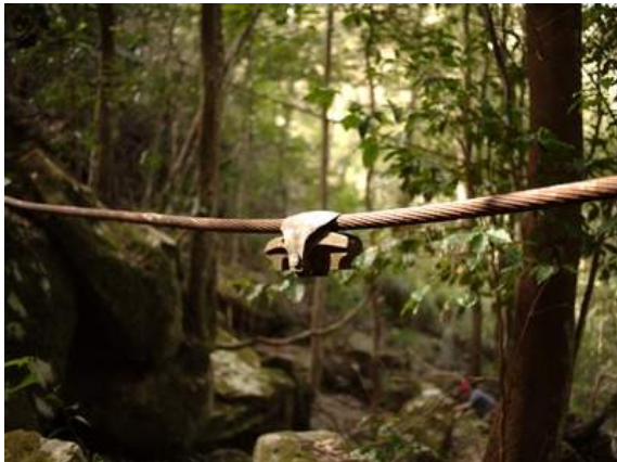
Figure 4.22 Some ropes remain suspended, having been caught on trees as they fell. This one has a saddle still in place. (Photo: P1020609)
