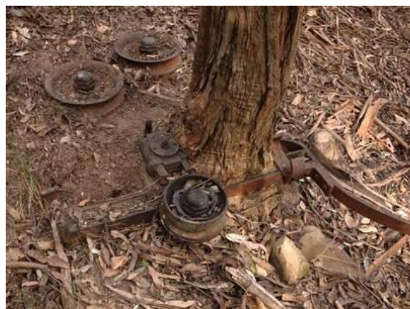
Figure 4.9 Carrier fixed in place by a tree trunk. (Photo P1070683)
